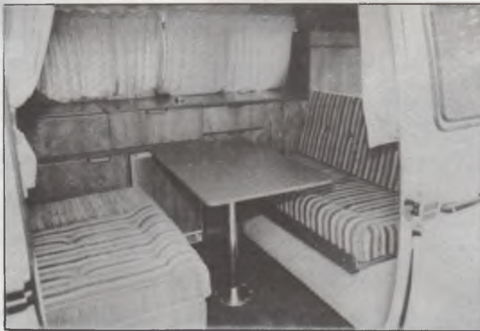
Fairly conventional layout, with kitchen on offside wall, face-forward settee and face-rearward occasional bench.
