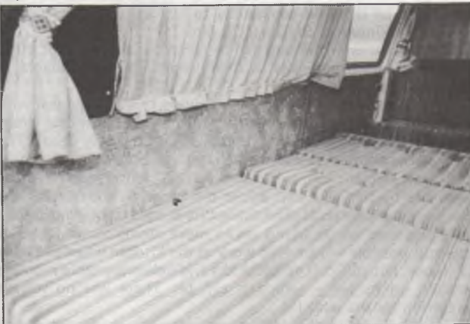
Side curtains have wire restrainers to hold them against windows. Wall beneath is cork-effect hardboard.
