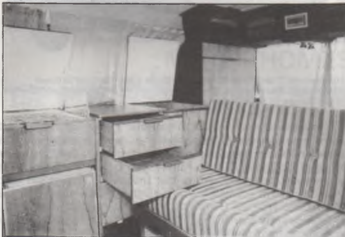
Sink and cooker, left of photo, frig beneath. Lower of two drawers comes right out to reveal hidden locker.
