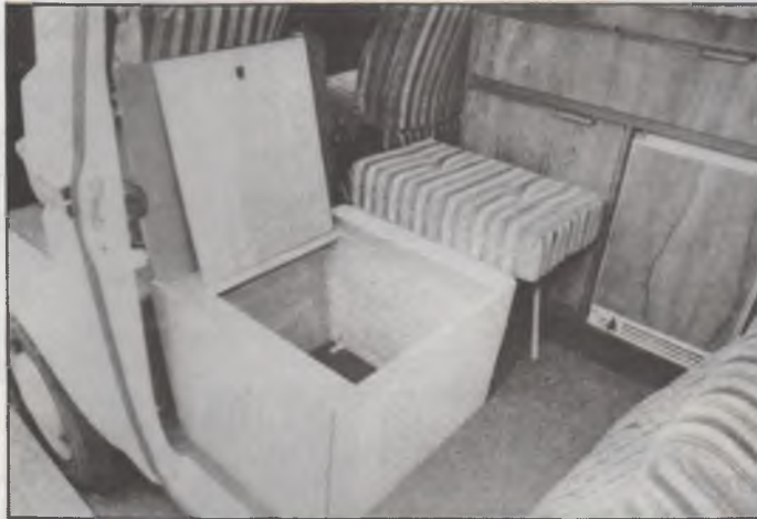
Single seat behind cab will take Porta-Potti in base. Fourth seat, based on hinged flap, spans gangway.
