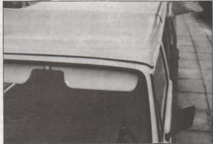
No need to unload roofrack before raising roof. Production models will have cleats for luggage straps.
